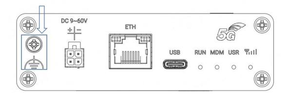
**5. Connect the router to the computer.** Connect the Ethernet cable to any port labeled ETH of the router, and connect the other end of the cable to your computer.
