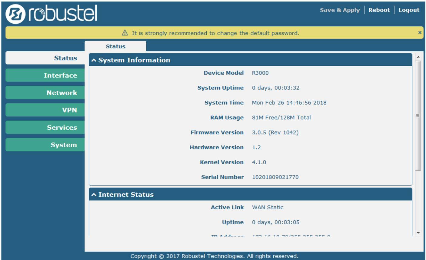
Using the original password to log in the router, the page will pop up the following tab
