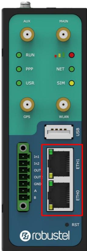
There are two Ethernet ports on R3000 Router, including ETH0 and ETH1. Each Ethernet port has two LED indicators. The yellow one is a link indicator, while the green one is a speed indicator. For details about status, see the table below.
