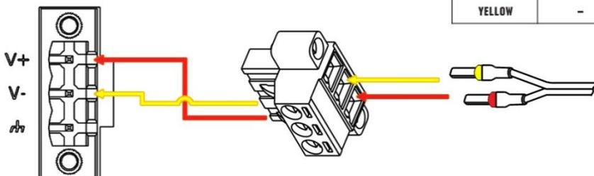
R3000 Router supports reverse polarity protection, but always refers to the figure above to connect the power adapter correctly. There are two cables associated with the power adapter. Following to the color of the head, connect the cable marked red to the positive pole through a terminal block, and connect the yellow one to the negative in the same way. The last step is to plug the power adapter into your socket.
