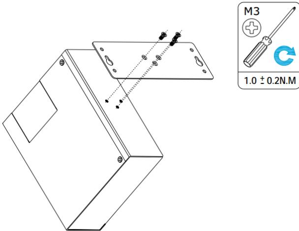
Use 3 pcs of M3\*4 flat head Phillips screws to fix the wall mounting kit to the router, and then use 2 pcs of M3 drywall screws to mount the router associated with the wall mounting kit on the wall.
