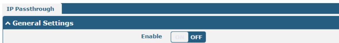
If router enables the IP Pass-through, the terminal device (such as PC) will enable the DHCP Client mode and connect to LAN port of the router; and after the router dial up successfully, the PC will automatically obtain the IP address and DNS server address which assigned by ISP.
