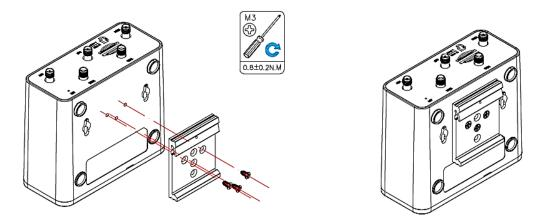
Use 3 pcs of M3\*8 Black cross recessed countersunk head tapping screws to mount the router on the DIN rail, and then hang the DIN rail on the holder. You need to choose a standard holder.
