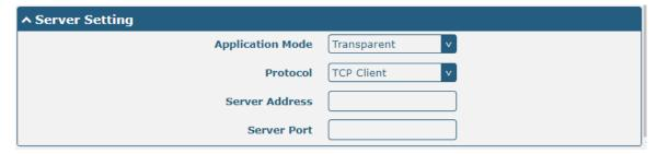
In the "Server Settings" column, when you select "Transparent Transmission" as the application mode and "TCP Client" as the protocol, the window is as follows:
