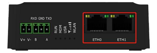
There are two Ethernet ports on R1511, including ETH0 (WAN/LAN), and ETH1. Each has two LED indicators. The green one is a link indicator but the yellow one doesn't mean anything (always off). For details about status, see the table below.
