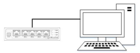
Connect the router's Ethernet port (ETH0~ETH4) to a PC with a standard Ethernet cable.
