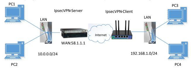
IPsec VPN topology (server-side and client-side IKE and SA parameters must be configured the same).
