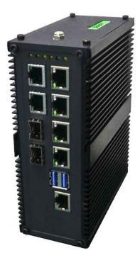
The DIN-Rail Industrial PC is a small form factor fanless embedded computer which supports wide temperature for 24/7 industrial application environments.
